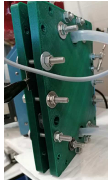
BDD anode SS cathode
