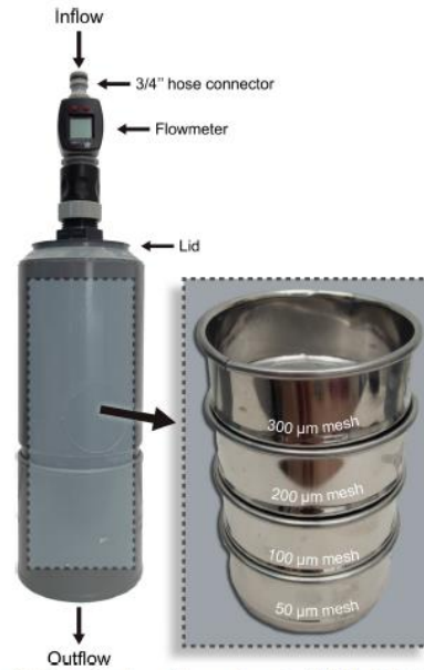
Fig 2. Sampling device diagram. The pump underway system of the RV Ángel Albariño had a tap connection at the wet lab to which the filtering device was connected with a 3/4" hose. This figure shows real pictures of the sampling device used in this study, with the stacked sizes that it contains shown on the right.
